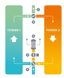
The main air flow is now dried by Tower 2 while Tower 1 is being regenerated.
